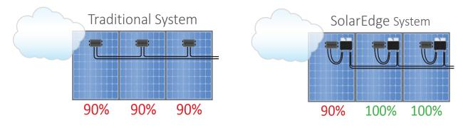
SolarEdge further increases FiT revenue by minimising energy loss due to panel aging. Panel performance degrades over 20-25 years of operation, and since each panel ages at a different rate, mismatch between panels will increase over time.
